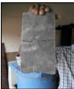
Fig 3 Specimen after Flexural strength
