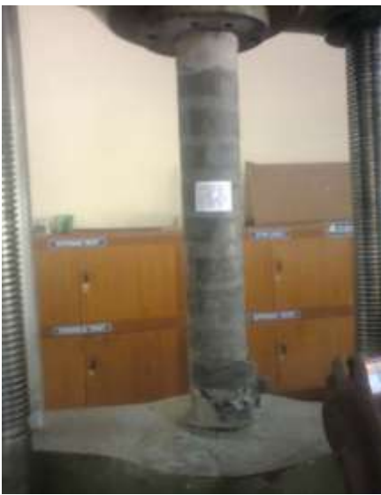
Fig 8. Failure mode of CFRP confined column specimen
