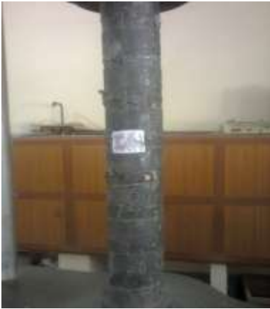
Fig 7. Testing of CFRP confined column specimen
