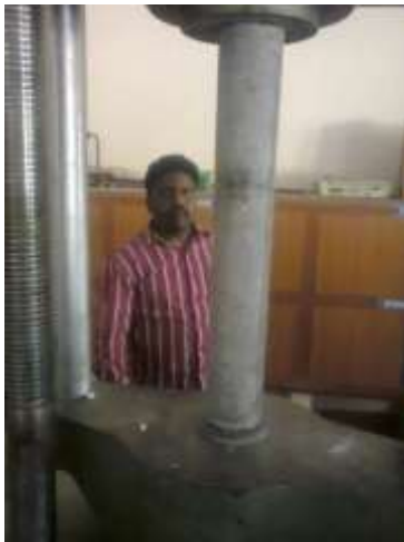
Fig 5. Testing of column
