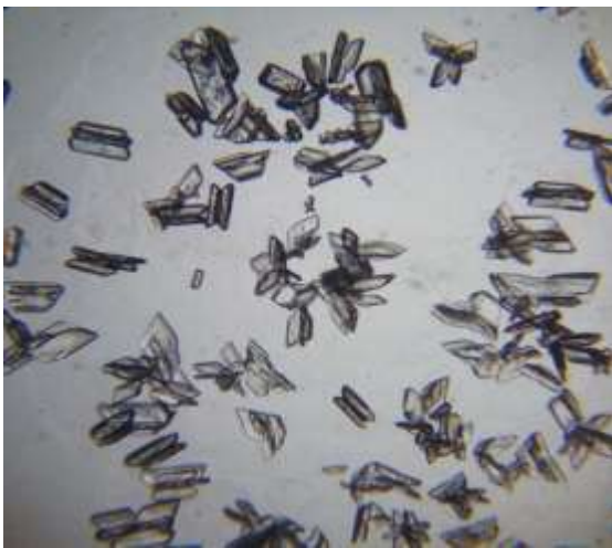
Figure 7 A: Microscopic view of Struvite crystals in Control Gel medium
