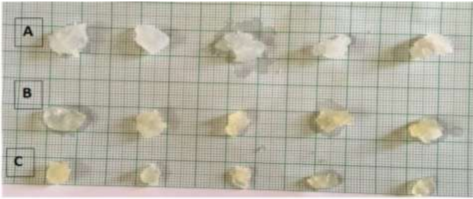
Figure 6: Size variation of Struvite crystals in control and EESE treated Medium
