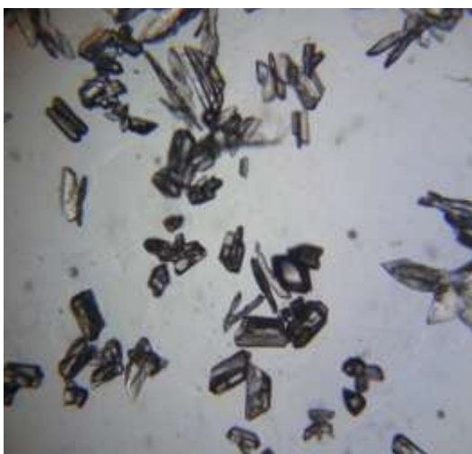
Figure 9 A: Microscopic view of Struvite crystals in Control Gel medium
