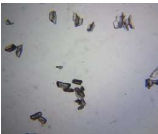
Figure 9 B: Microscopic view of Struvite crystals in 0.5% EESE treated medium
