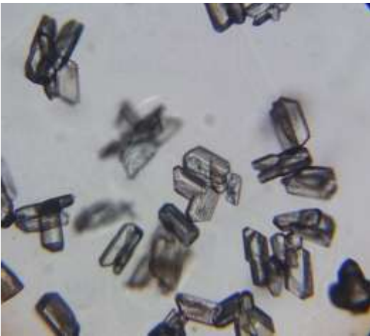
Figure 8 A: Microscopic view of Struvite crystals in Control Gel medium
