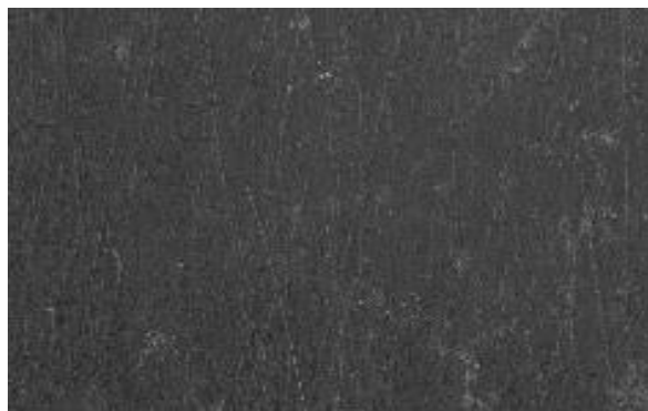
Figure 8. The SEM micrograph for mild steel in 1.0 M HCl with 0.5 mM of coumarin-3-amine at 30 °C for 5 h as immersion time.
