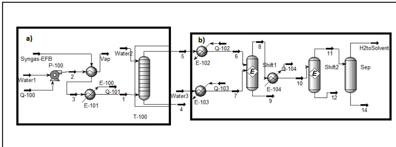
**Figure 3. Heat recovery, gas cleaning, LTS (Low Temperature Shift) reactors, HTS (High Temperature Shift) and decanter stages.**
