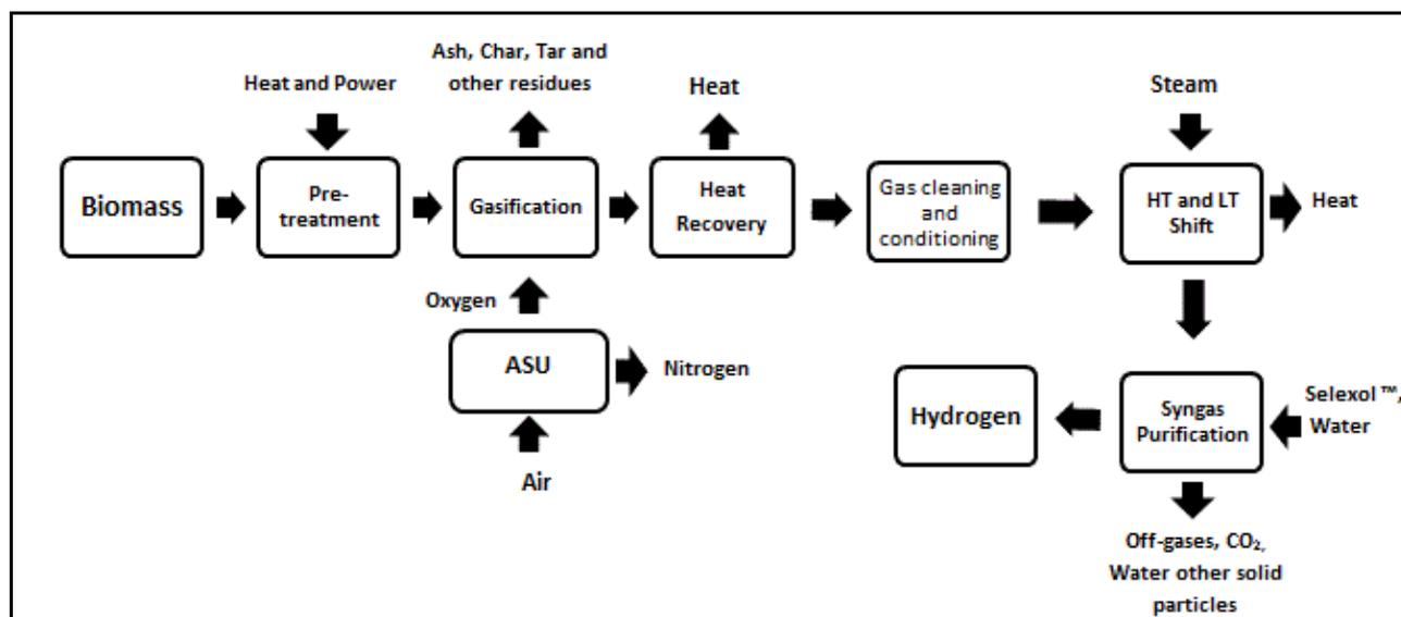
**Figure 1. Schematic model of the gasification based hydrogen production**
