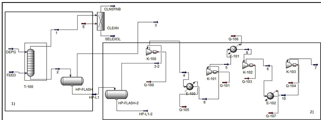
Figure 5. Syngas purification process using Selexol™ as solvent.
