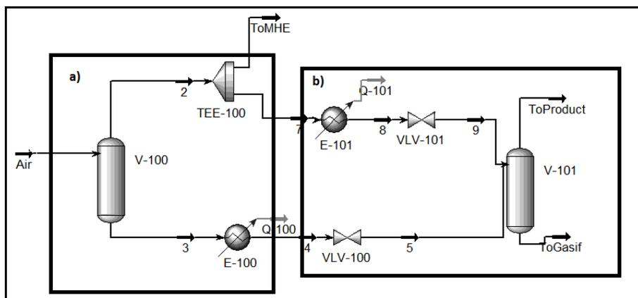
**Figure 2. HP (High pressure) and LP (Low pressure) column system of ASU cryogenic air distillation unit.**
