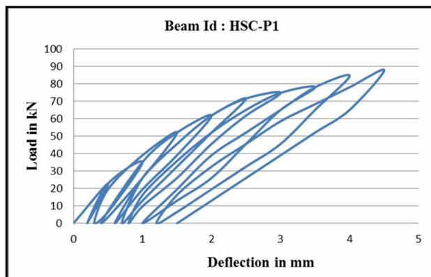
**Fig. 4(a) Cyclic Response of HSC-P1 Beam**
