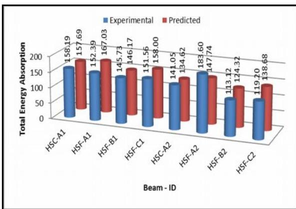
Fig. 16 Total Energy Absorption -Experimental Vs Predicted
