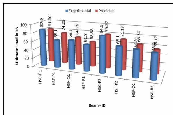
Fig. 13 Ultimate Load - Experimental Vs Predicted
