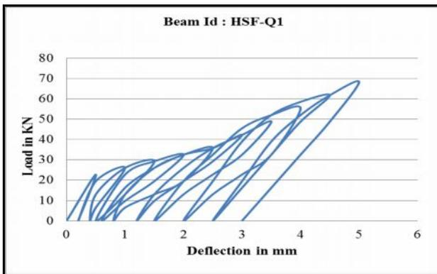
Fig. 4(e) Cyclic Response of HSF-Q1 Beam
