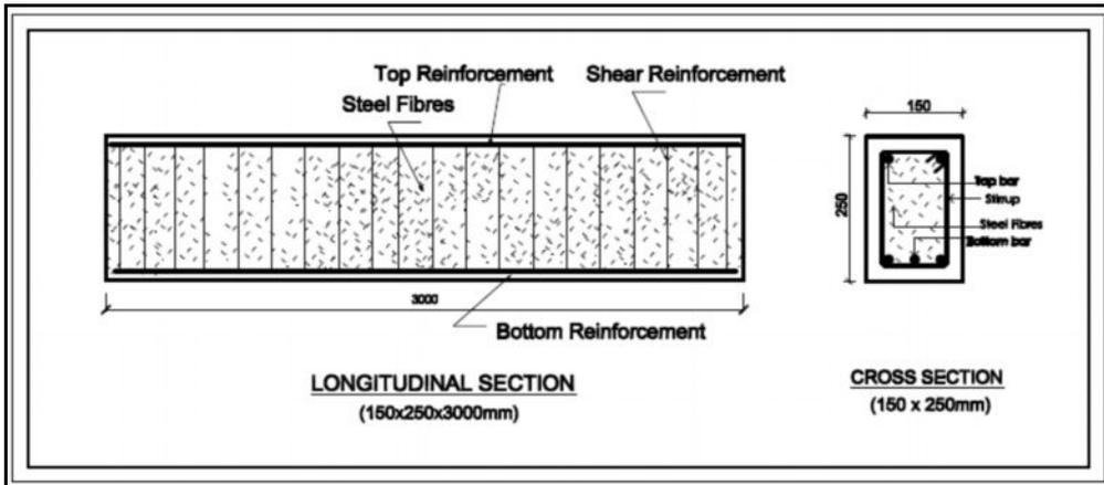
Fig.1. Reinforcement Details of Test Beam
