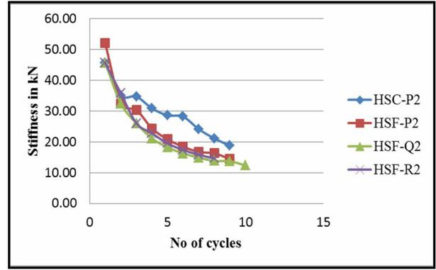
**Fig.8 Stiffness Vs No. of Cycles -200mm stirrup spacing**
