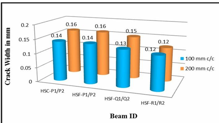
**Fig.11 Crack Width at Ultimate Stage**
