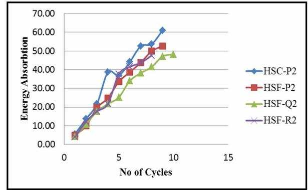
**Fig.10 Energy Absorption Vs No. of Cycles-200mm stirrup**
