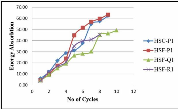
**Fig.9 Energy Absorption Vs No.of Cycles-100mm stirrup**
