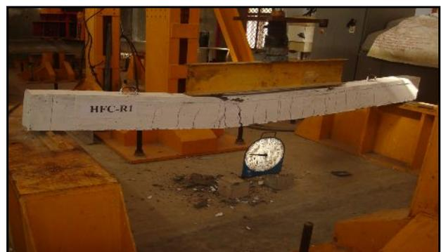
Fig. 3 Beams under cyclic load testing
