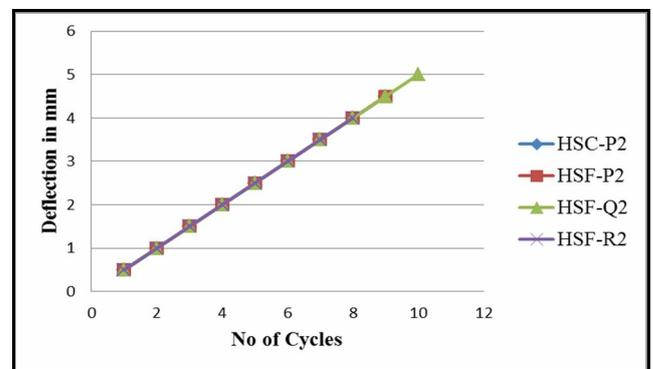
Fig. 6 Deflection Vs No. of Cycles -200mm stirrup spacing
