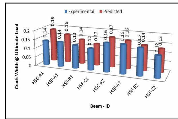
Fig.17 Crack Width at Ultimate Load- Experimental Vs Predicted
