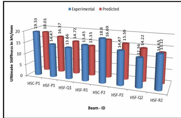
Fig. 15 Ultimate Stiffness - Experimental Vs Predicted
