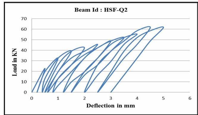
Fig. 4(f) Cyclic Response of HSF-Q2 Beam
