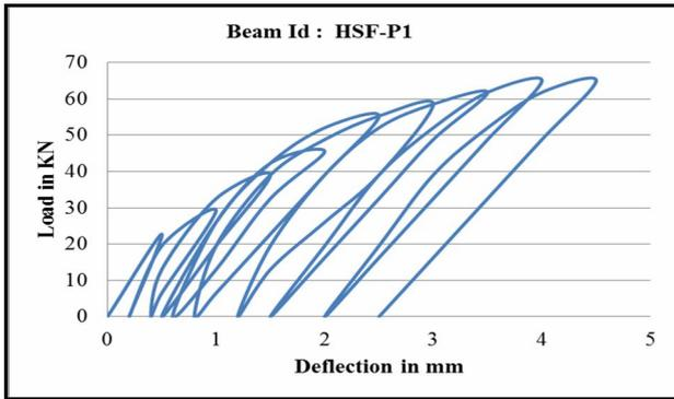
Fig. 4(c) Cyclic Response of HSF-P1 Beam
