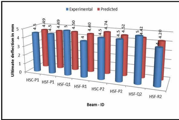
Fig. 14 Ultimate Deflection - Experimental Vs Predicted
