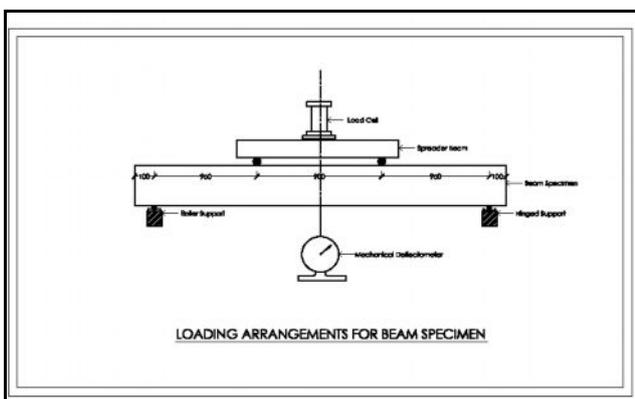
Fig. 2 Beam Test Setup Showing Details of Instrumentation
