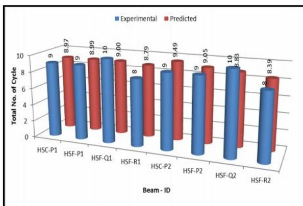
Fig.12 Total Number of Cycles - Experimental Vs Predicted
