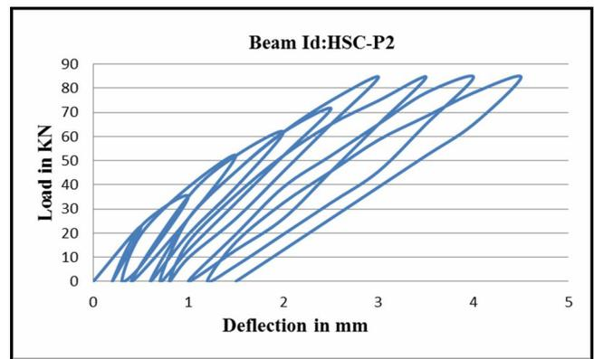
**Fig. 4(b) Cyclic Response of HSC-P2 Beam**
