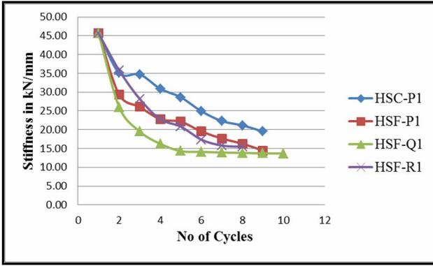
**Fig.7 Stiffness Vs No. of Cycles -100mm stirrup spacing**
