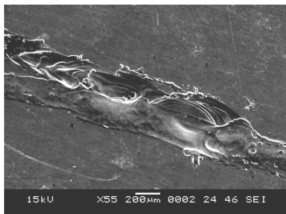
Figure3a Side 1–Stripe of non-uniform melted porosity in non-uniform melted tin
