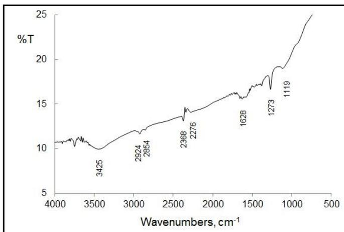
**Figure 7. FTIR spectra of silver nanoparticles. [*p*-hydroxybenzoic acid] =  $1.0 \times 10^{-3}$  M, [ $\text{AgNO}_3$ ] =  $2.0 \times 10^{-4}$  M, pH = 11**
