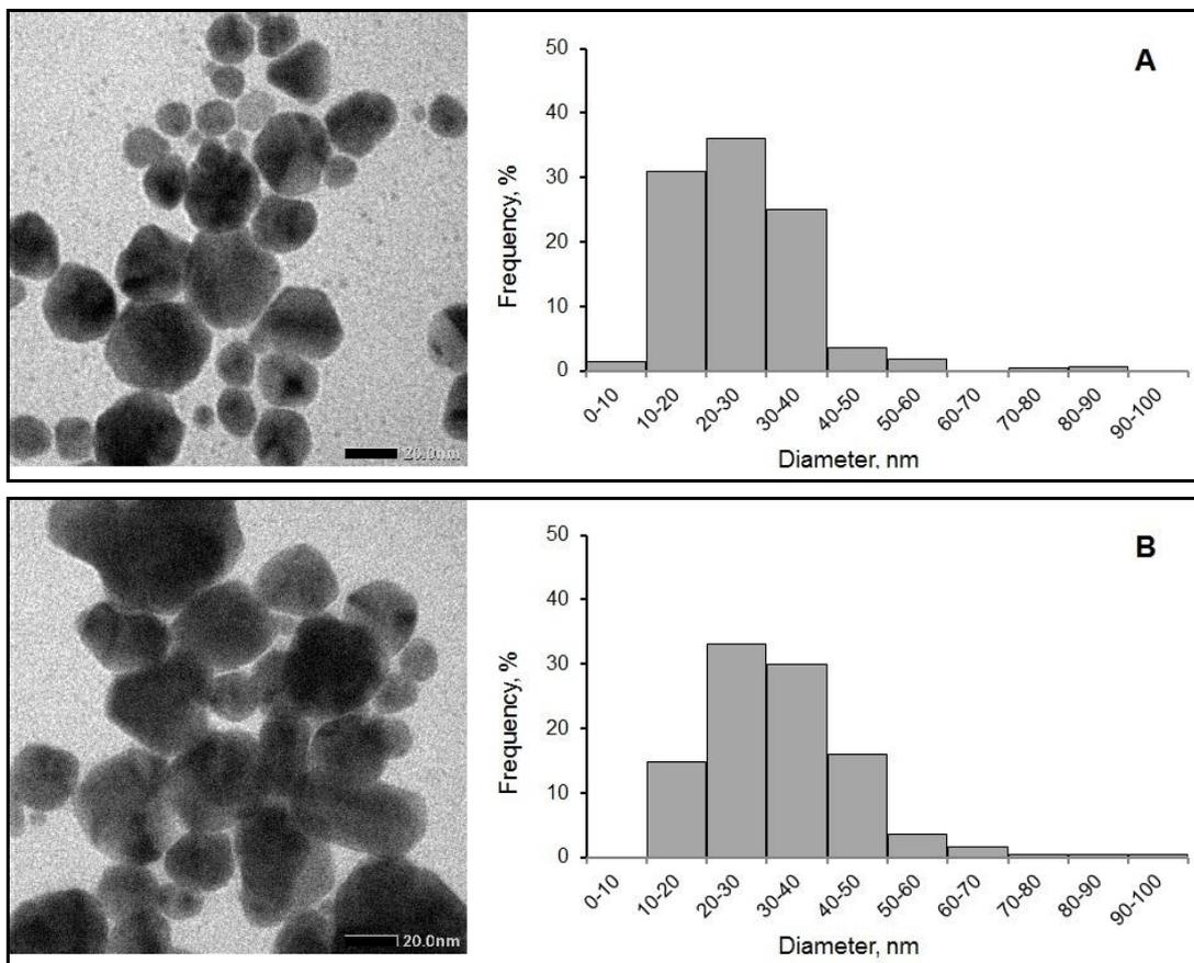
**Figure 5. TEM image and particle size distribution of resulting silver nanoparticles. Scale bar 20 nm, (A). Mole ratio of  $\text{AgNO}_3$ :*p*-hydroxybenzoic acid 1:20 (B). Mole ratio of  $\text{AgNO}_3$ :*p*-hydroxybenzoic acid 1:50**
