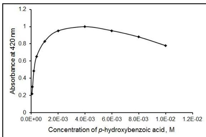
**Figure 3.** Plot of silver nanoparticles absorbance at 420 nm and concentration of *p*-hydroxybenzoic acid used in formation of silver nanoparticles. [*p*-hydroxybenzoic acid] =  $0.5 \times 10^{-4}$ – $1.0 \times 10^{-2}$  M, [ $\text{AgNO}_3$ ] =  $2.0 \times 10^{-4}$  M, pH = 11
