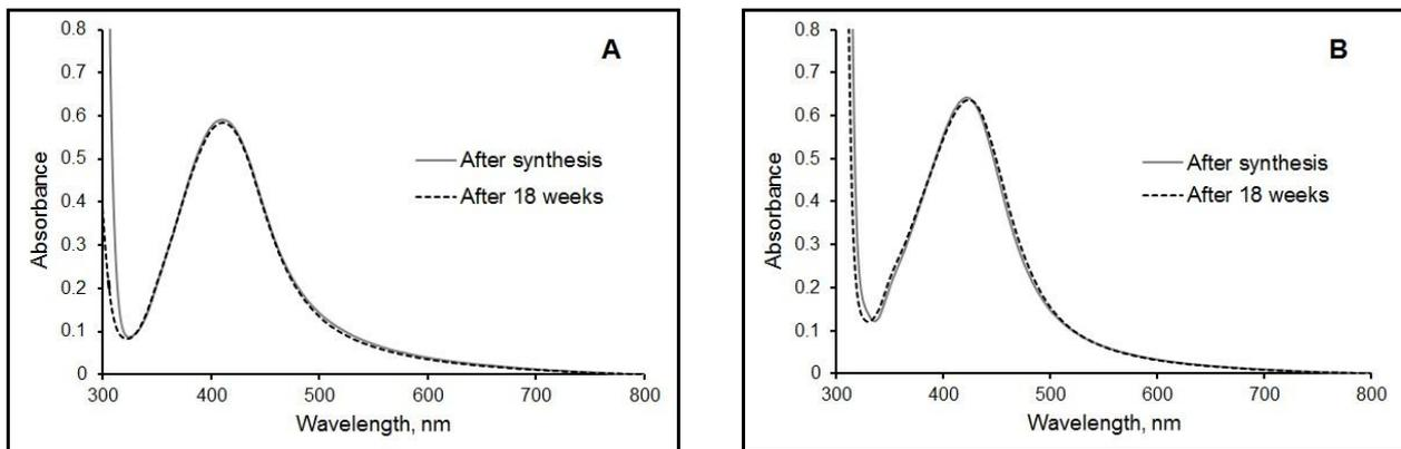
**Figure 6. UV-visible spectra of silver nanoparticles after a period of 18 weeks. (A). [*p*-hydroxybenzoic acid] =  $1.0 \times 10^{-3}$  M, [ $\text{AgNO}_3$ ] =  $1.5 \times 10^{-4}$  M, pH = 11, (B). [*p*-hydroxybenzoic acid] =  $1.0 \times 10^{-2}$  M, [ $\text{AgNO}_3$ ] =  $1.5 \times 10^{-4}$  M, pH = 11,**
