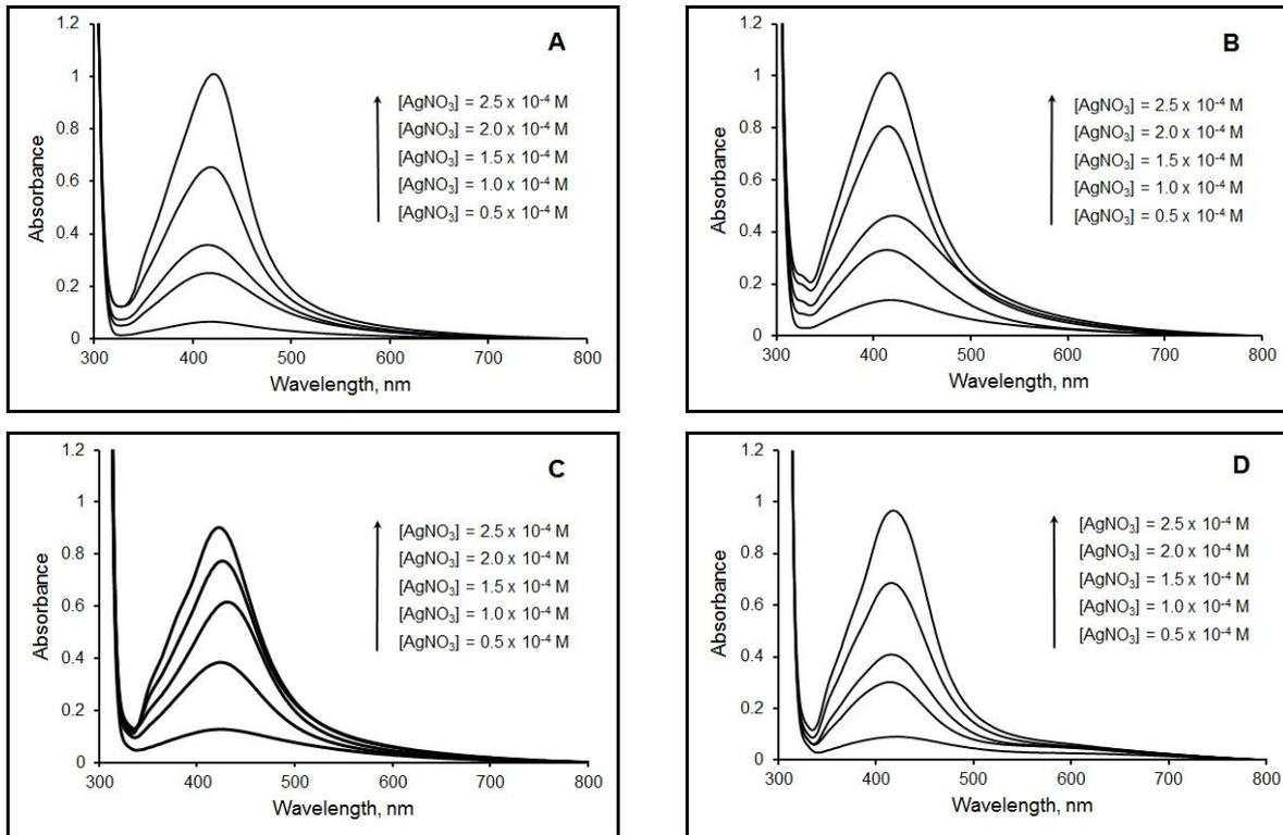
**Figure 2.** UV-visible spectra of silver nanoparticles using different initial concentration of  $\text{AgNO}_3$ .  $[\text{AgNO}_3] = 0.5\text{-}2.5 \times 10^{-4}$  M, (A). [*p*-hydroxybenzoic acid] =  $1.0 \times 10^{-3}$  M, pH = 11, (B). [*p*-hydroxybenzoic acid] =  $1.0 \times 10^{-3}$  M, pH = 12, (C). [*p*-hydroxybenzoic acid] =  $1.0 \times 10^{-2}$  M, pH = 11, (D). [*p*-hydroxybenzoic acid] =  $1.0 \times 10^{-2}$  M, pH = 12
