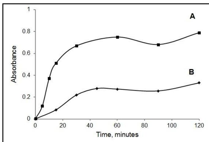
**Figure 1. Reaction time of silver nanoparticles formation (A).** [*p*-hydroxybenzoic acid] =  $1.0 \times 10^{-3}$  M, [ $AgNO_3$ ] =  $2.0 \times 10^{-4}$  M, pH = 11, (B). [*o*-hydroxybenzoic acid] =  $1.0 \times 10^{-2}$  M, [ $AgNO_3$ ] =  $3.0 \times 10^{-4}$  M, pH = 11
