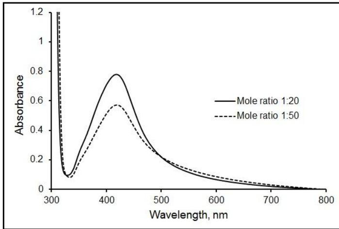
**Figure 4. UV-visible spectra of silver nanoparticles resulted from reaction with different mole ratio of  $\text{AgNO}_3$  to *p*-hydroxybenzoic acid**
