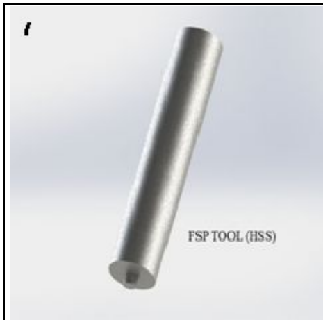
Fig:3.1:(a) The design geometry FSP tool
