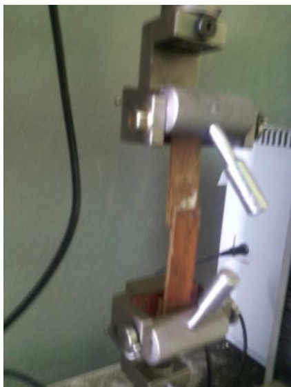
Figure 3.4 Single lap joint wood specimen clamped by the knurled jaw for testing
