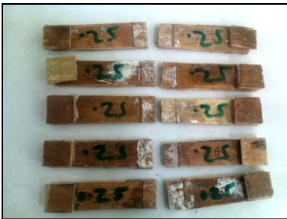
Figure 3.1 Results of 0.25mm bond line thickness and lap length 10mm specimen after bond failure
