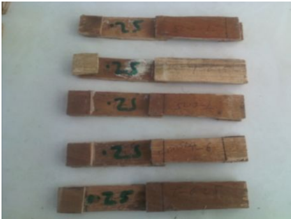
Figure 2.3Single lap joint wood specimen after shim and spacer removal before test
