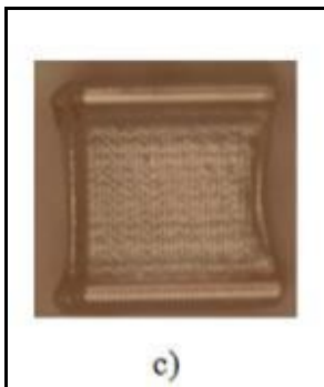
Fig.5 a) The principle of microstereolithography[13], b) HDAA sample CAD model, c) Optical microscope picture of the sample (0.5 X 0.5 X 0.7 mms).
