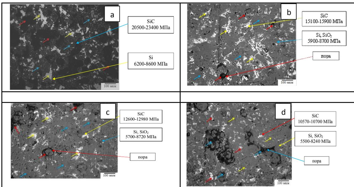
**Fig: (3).** Microstructure of surface of the obtained samples at micro-hardness at different areas a) prototype of the siliconized graphite b) with mass ratios of 70 % SiO<sub>2</sub> and 30% C; c) with mass ratios of 40 % SiO<sub>2</sub> and 60 % C; d) with mass ratios of 60 % SiO<sub>2</sub> and 40% C
