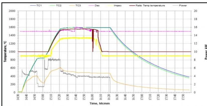
Fig: (1). Temperature heating mode of the samples
