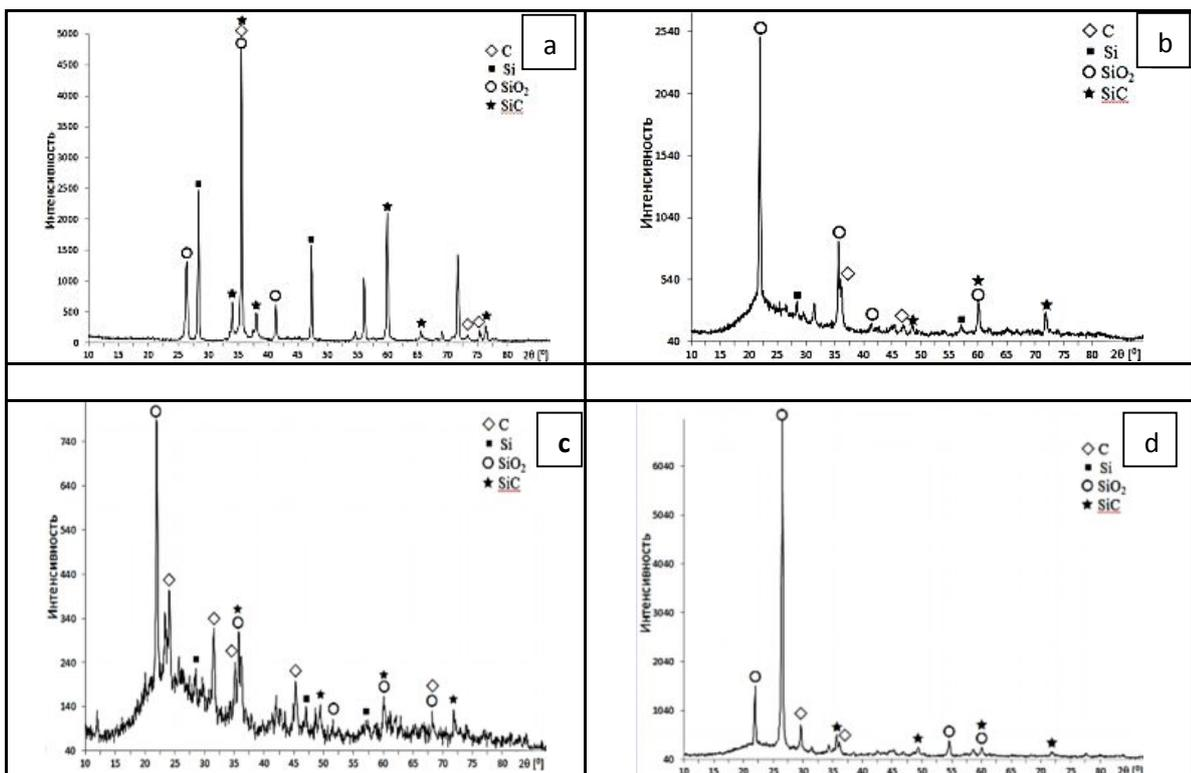
**Fig: (4).** X-ray phase diffractogram of the test the samples a) a prototype of the siliconized graphite b) with a mass ratios of 70 % SiO<sub>2</sub> and 30 % C; c) with a mass ratios of 40 % SiO<sub>2</sub> and 60 % C; d) with a ratios of 60 wt% SiO<sub>2</sub> and 40 % C
