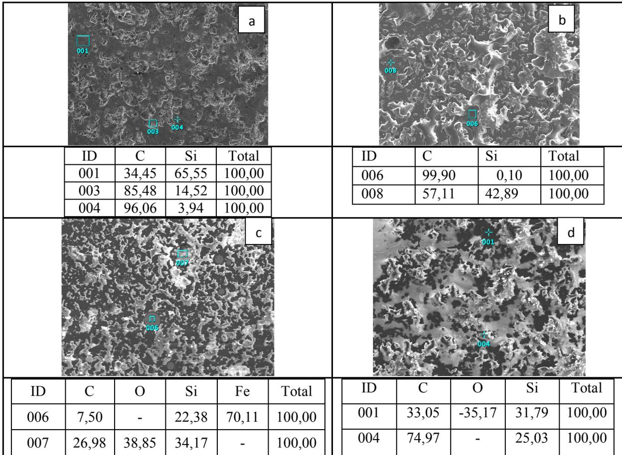
**Fig: (5). Results of EDS-analysis. The distribution of elements in wt.% a) the prototype of the siliconized graphite b) with mass ratios of 70 % SiO<sup>2</sup> and 30 % C; c) with mass ratios of 40 % SiO<sub>2</sub> and 60 % C; d) with mass ratios of 60 % SiO<sub>2</sub> and 40 % C**
