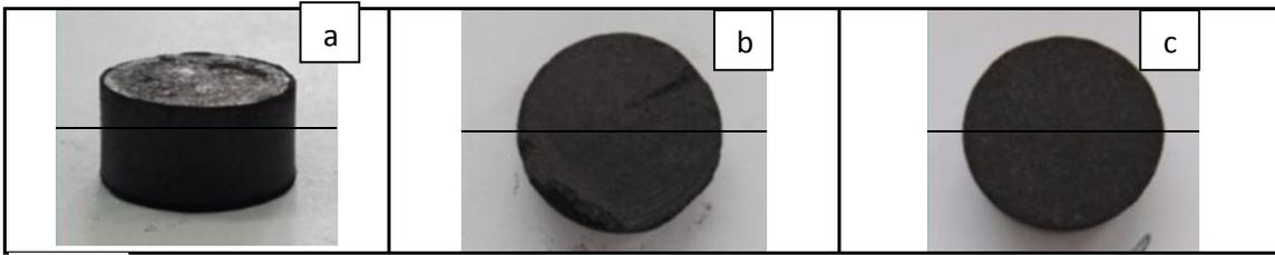
**Fig: (2).** The test samples after sintering at a temperature of 1550 a) with a mass ratios of 70 % SiO<sub>2</sub> and 30% C; b) with mass ratios of 40 % SiO<sub>2</sub> and 60 % C; c) with mass ratios of 60 % SiO<sub>2</sub> and 40 % C
