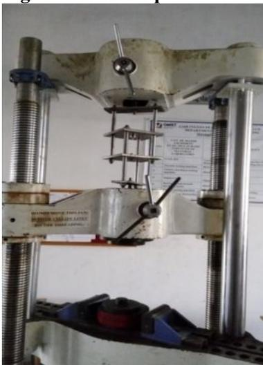
**Fig. 5 Universal Testing Machine clamped with Miniature Specimen**
