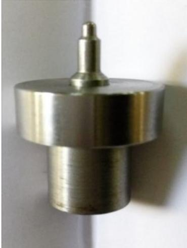
**Fig. 3 Punch in a punch holder**
