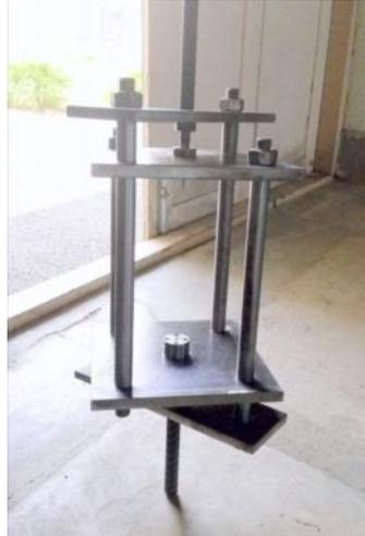
**Fig. 4 Small punch test fixture**
