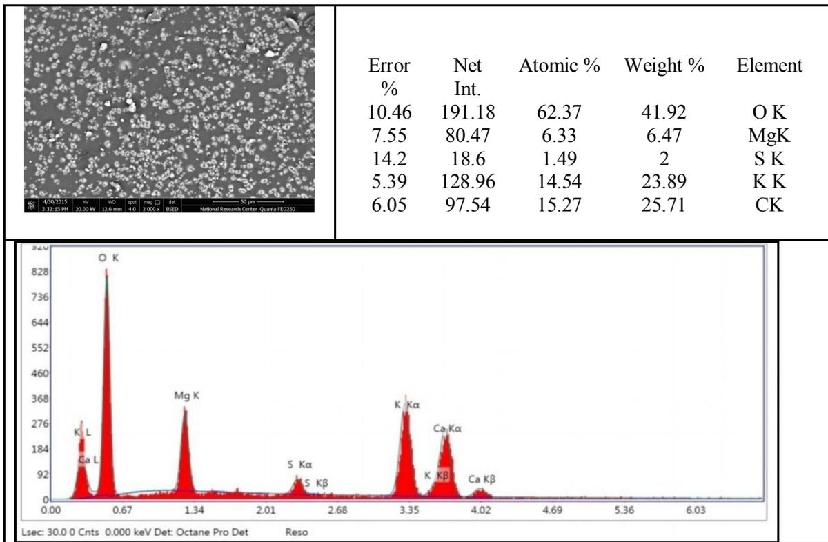
Figure 7: SEM & EDAX analysis of SAH loaded with 0.4 % MgO nanoparticles.
