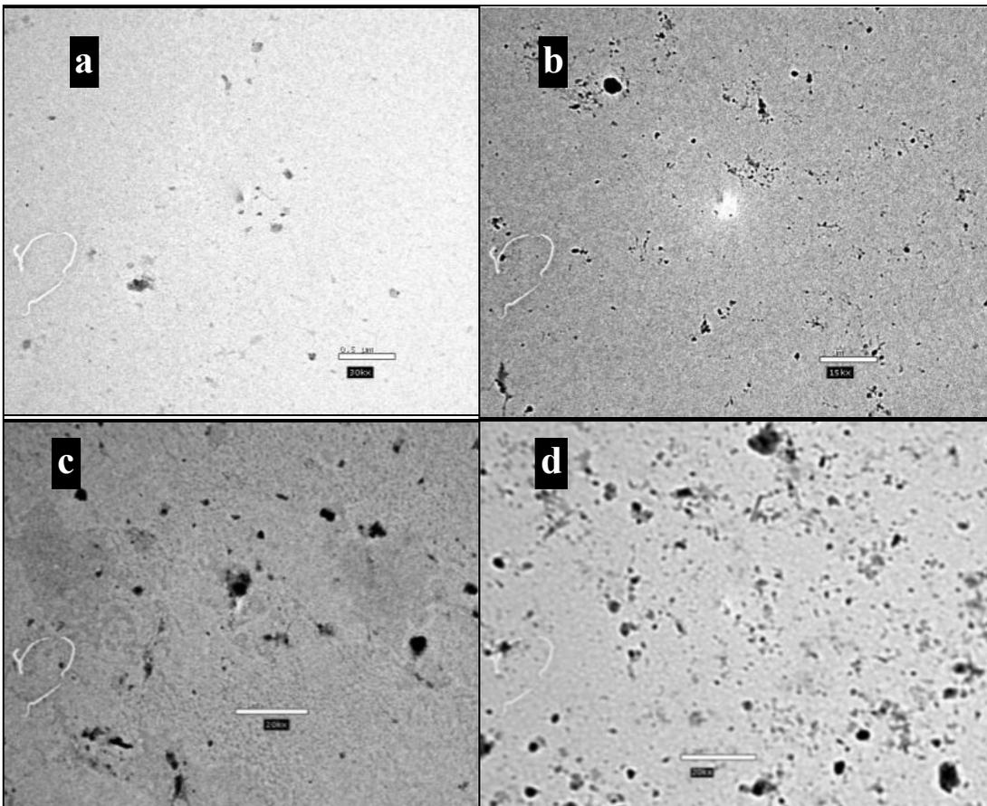
Figure 1: TEM images of the PAAC/AC hydrogel loaded with different amounts of magnesium oxide Nanoparticles (a) 0.1% MgO (b) 0.2% MgO (c) 0.3% MgO (d) 0.4% MgO.
