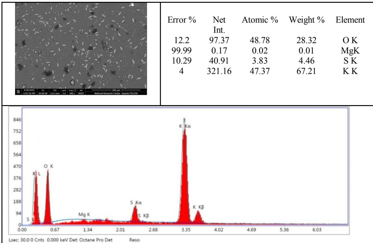
Figure 4: SEM & EDAX analysis of SAH loaded with 0.1 % MgO Nanoparticles.
