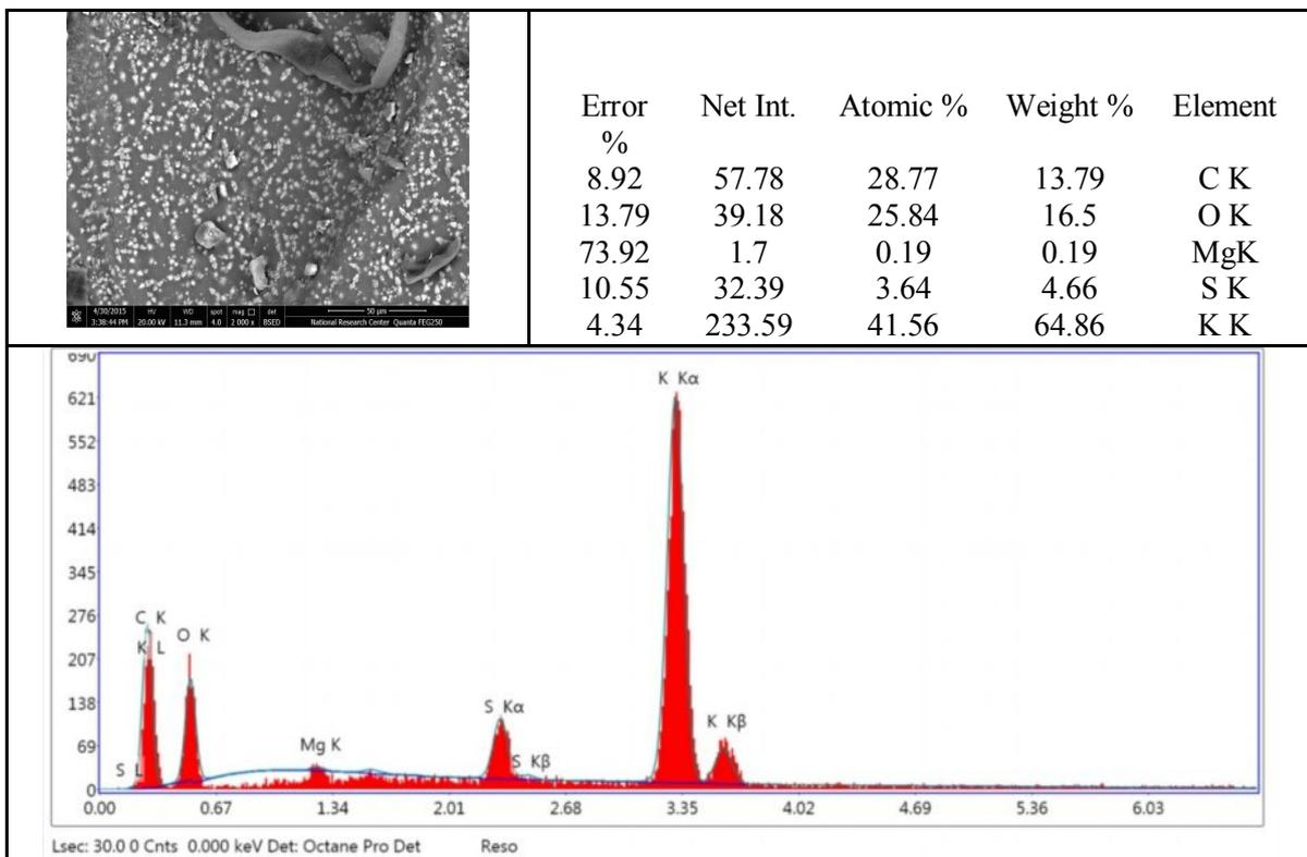
Figure 6: SEM & EDAX analysis of SAH loaded with 0.3 % MgO Nanoparticles.
