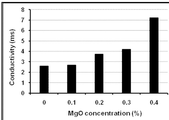
Figure 8: Conductivity of PAAc/Acrylate loaded with variable amounts of MgO.
