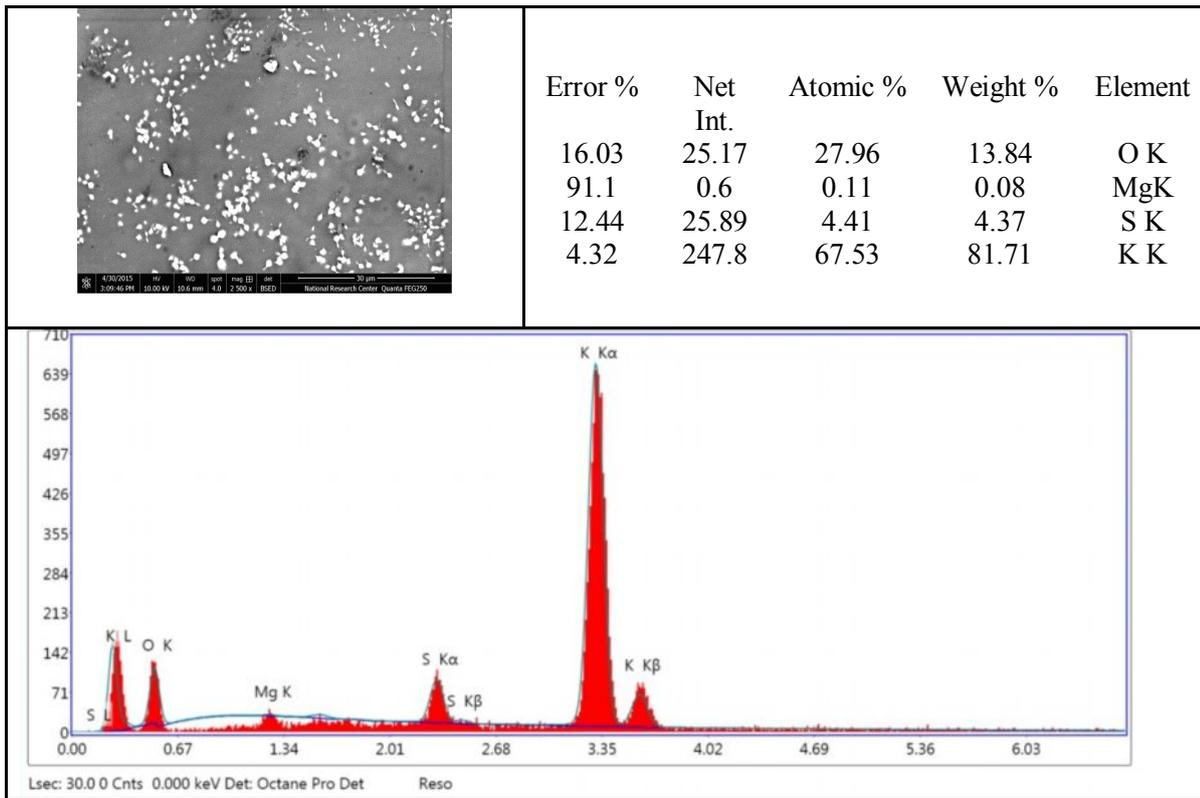
Figure 5: SEM & EDAX analysis of SAH loaded with 0.2 % MgO Nanoparticles.
