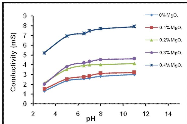
Figure 9: Effect of swelling pH on SAH conductivity
