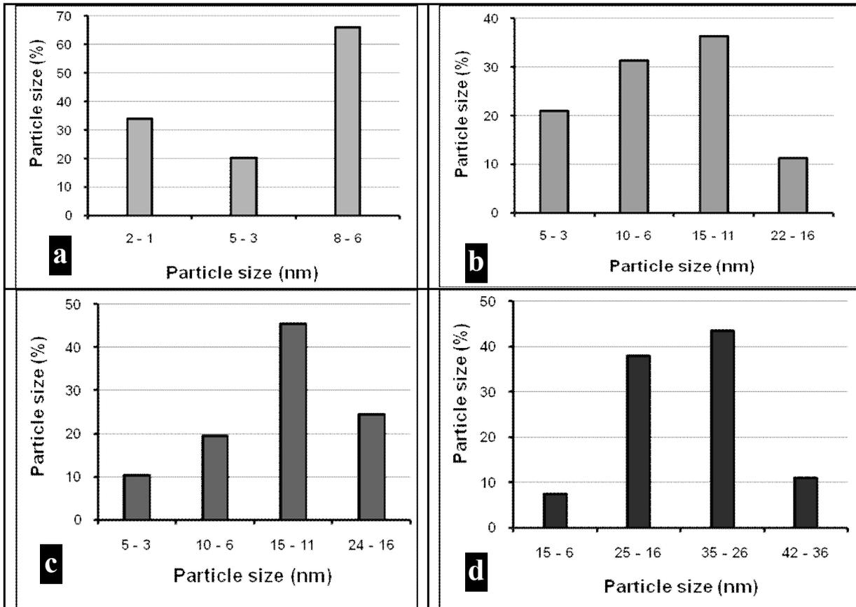
**Figure 2: Histogram of MgO Nanoparticles distribution within SAH matrix related to MgO dose (a) 0.1%; (b) 0.2%; (c) 0.3% and (d) 0.4%.**
