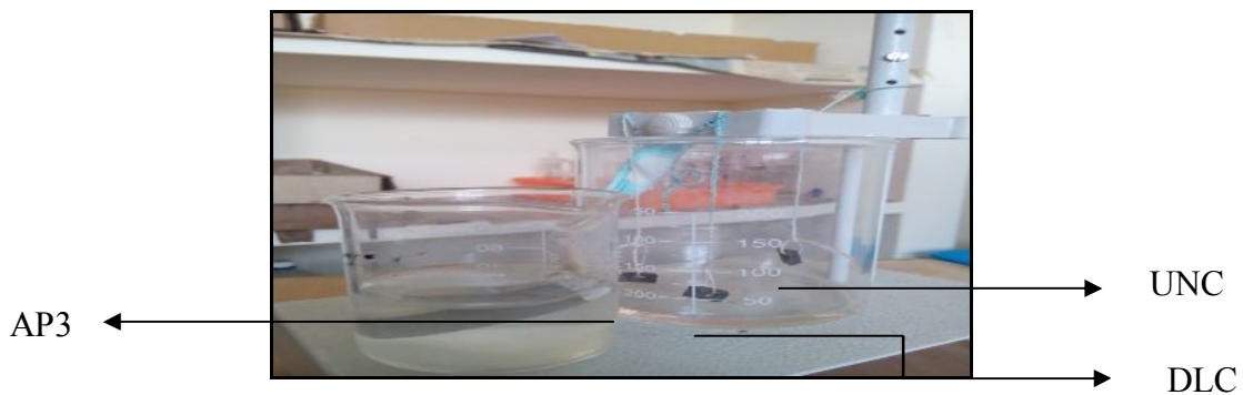
Fig 2 Arrangement of corrosion test on Acid medium
