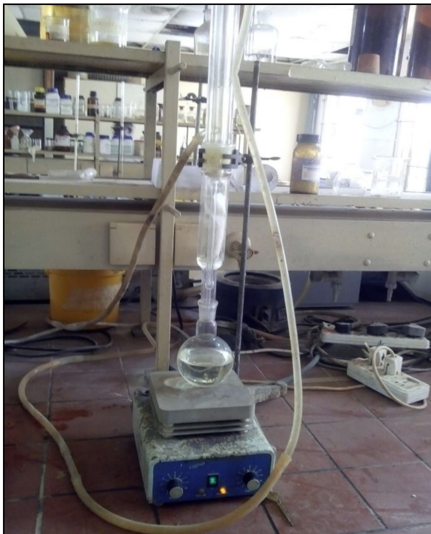
Figure 4. Experimental set-up for oil extraction
