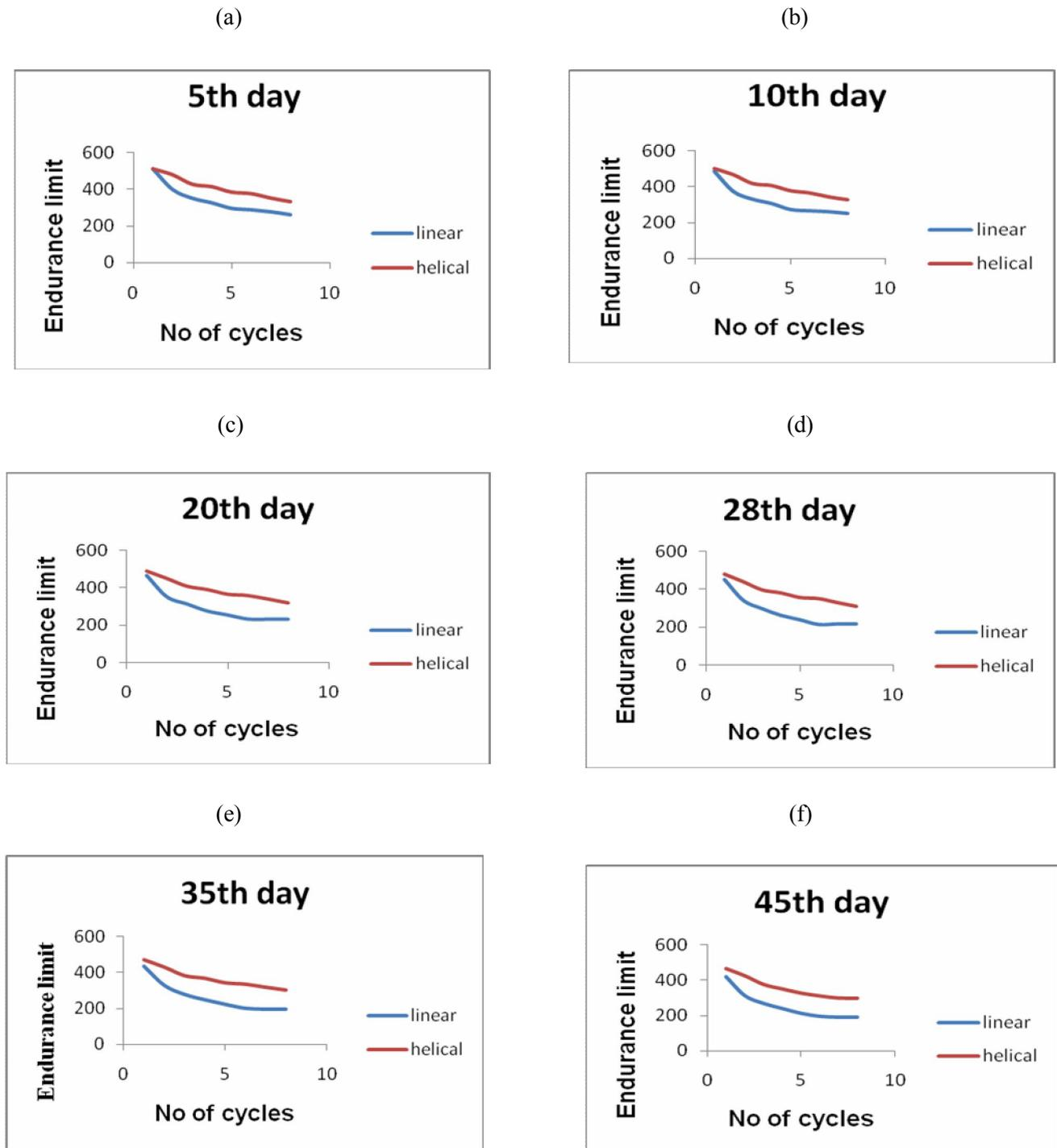
**Fig 3.2: Endurance limit variation of SS helical coil tube for various days of heating (a) 5th day (b) 10th day (c) 20th day (d) 28th day (e) 35th day (f) 45th day**
