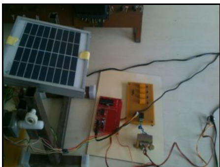
Fig.11: Movable solar tracking model
