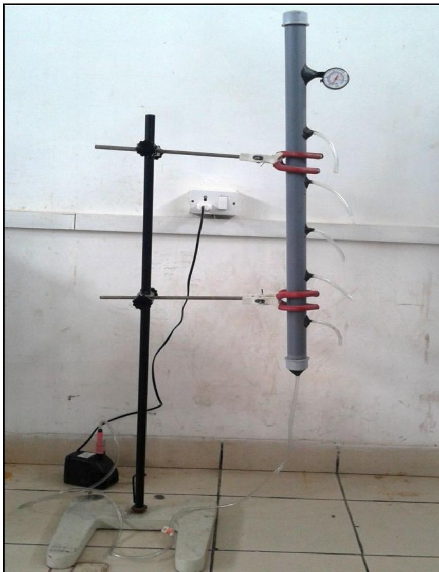
**Fig 3 Experimental setup of Continuous flow column**
