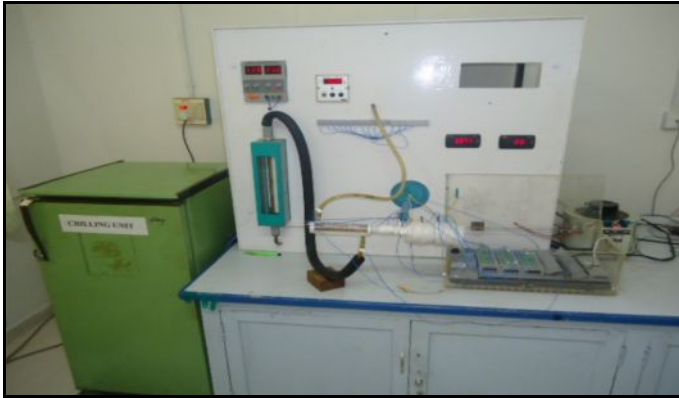
Fig 2. The experimental testing setup of the Heat pipe
