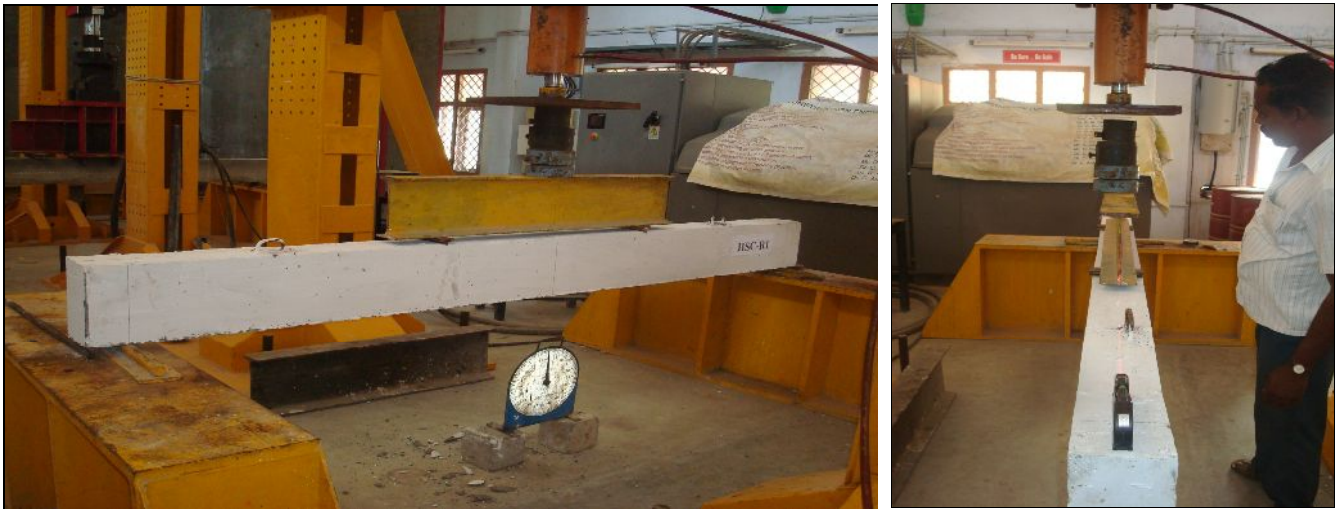
Fig. 2. Cyclic Load Beam Test Set-up
