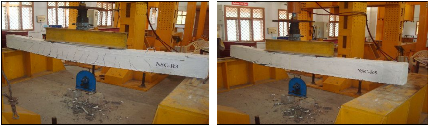
Fig. 12. Crack Patterns under Cyclic Loading
