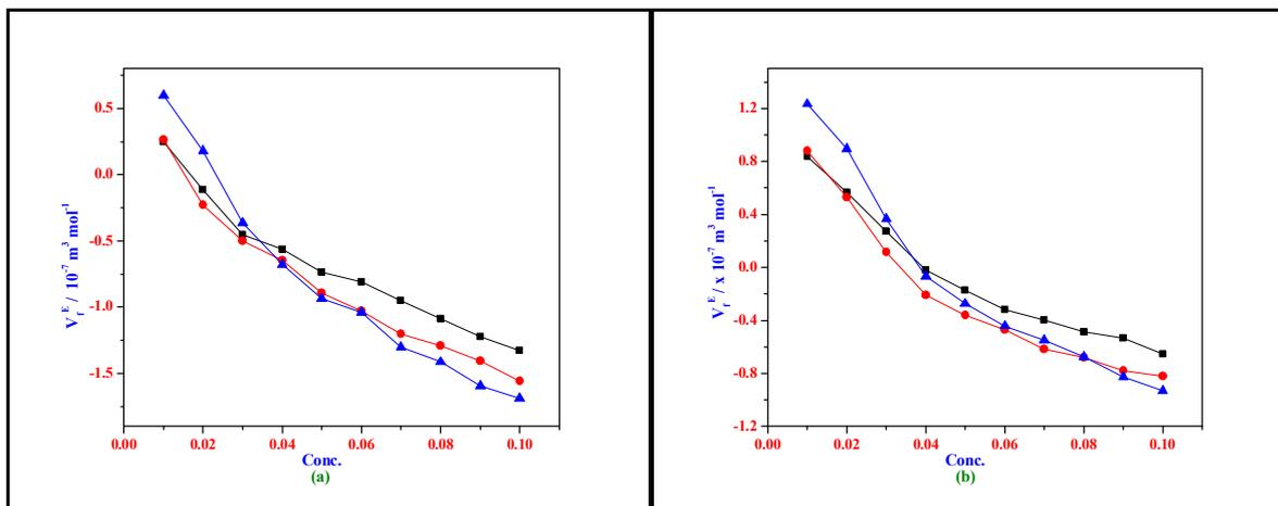
Figure 4 Plots of excess free volume versus concentration for a) Phenol and b) 4-ChP with NMA in n-hexane system at different temperatures (■) T = 293 K, (●) 298 K and (▲) 303 K
