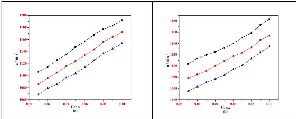
Figure 1 Plots of ultrasonic velocity versus concentration for a) Phenol and b) 4-ChP with NMA in n-hexane system at different temperatures (■) T = 293 K, (●) 298 K and (▲) 303 K
