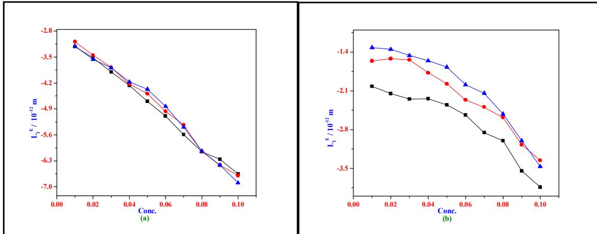
Figure 5 Plots of excess free length versus concentration for a) Phenol and b) 4-ChP with NMA in n-hexane system at different temperatures (■) T = 293 K, (●) 298 K and (▲) 303 K
