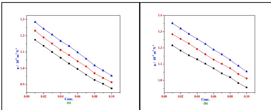
Figure 2 Plots of adiabatic compressibility versus concentration for a) Phenol and b) 4-ChP with NMA in n-hexane system at different temperatures (■) T = 293 K, (●) 298 K and (▲) 303 K
