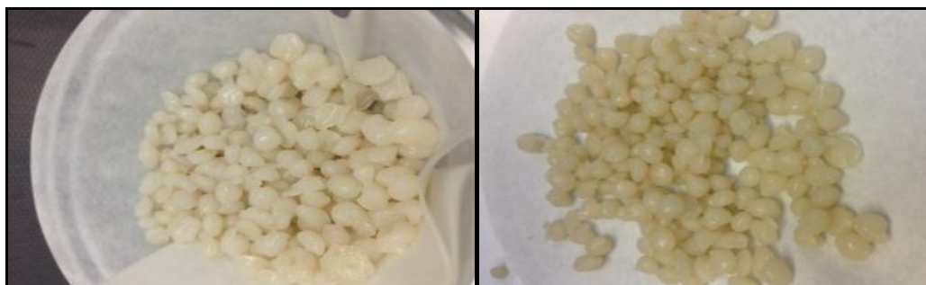
(Figure 6 a ,b) Immobilized cell with calcium alginate
