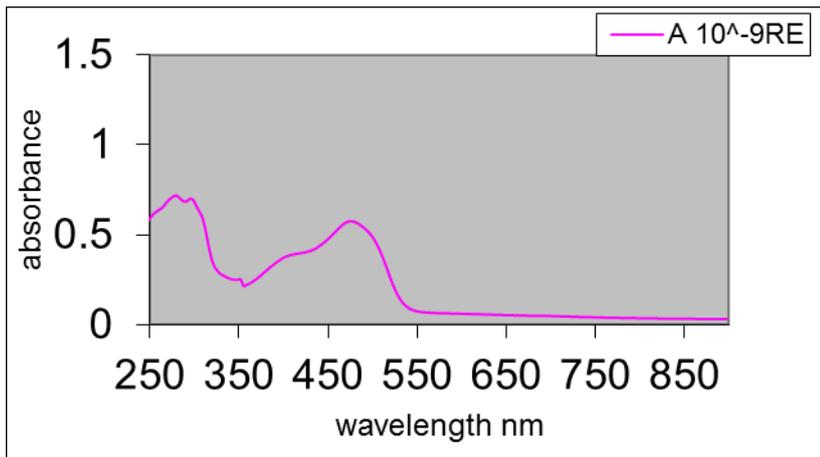
Figure (3) absorption spectral for Reactive Red ( $10^{-9}$  M)
