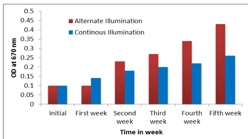
Figure 1: Growth of microalgae with reference to absorbance (OD) at 670 nm
