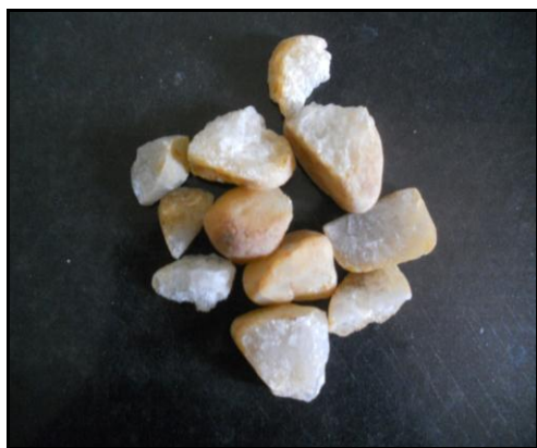
Fig. 2: Crushed Pebbles before TiO 2 coating.
