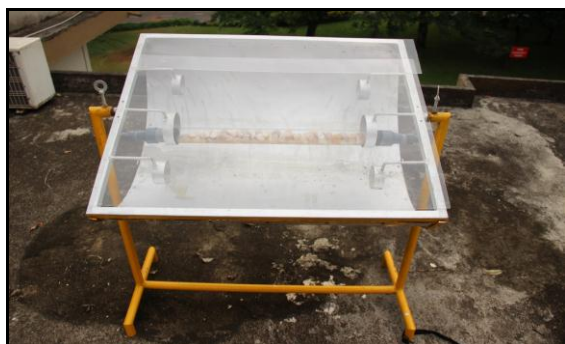
Fig. 5 : Pebble bed reactor setup for effluent treatment
