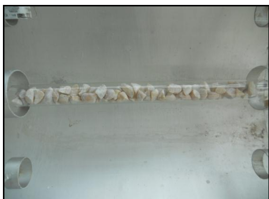
Fig. 4: Borosilicate tube filled with TiO 2 coated pebbles (Pebble column)
