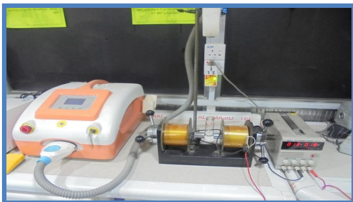
Figure 1 : The experimental setup preparation of nanoparticles by laser ablation process under the influence of a magnetic field.
