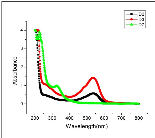
**Fig 2 Optical absorption of samples with dilution (D2) Beta vulgaris (D3) Punica granatum (D7) Tecoma Stans samples with dilution**
