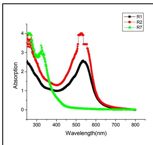
**Fig 1 Optical absorption of samples without dilution (R1) Beta vulgaris (R2) Punica granatum (R7) Tecoma Stans samples without dilution**
