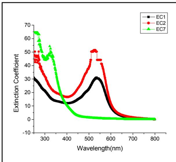
**Fig 3 Extinction coefficient Vs wavelength of (EC1) Beta vulgaris (EC2) Punica granatum (EC7) Tecoma Stans without dilution**
