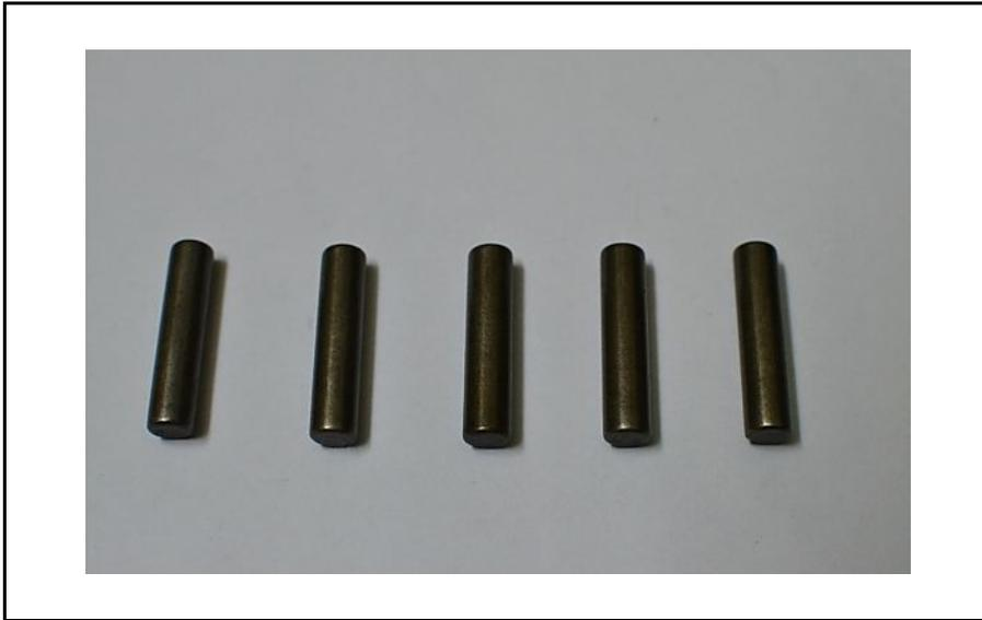
Figure 1 Photograph of a few chromized and treated samples
