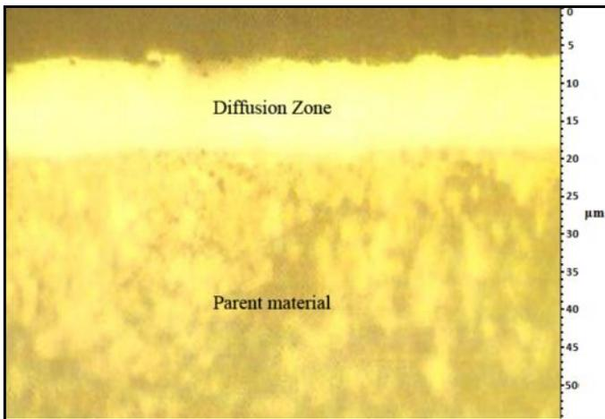
Figure 7Microstructure of the specimen chromized under optimal condition.
