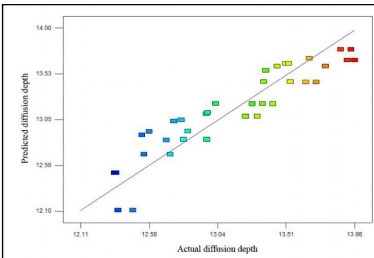
Figure 5 Plot of actual and predicted values of diffusion depth
