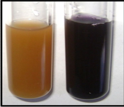
Figure 2: Test tubes containing bio-synthesized gold nanoparticles by Padina pavonica , a) before reaction and b) after 2 hours of reaction.
