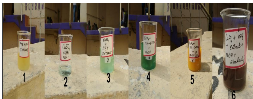
Fig.2: Photograph indicating the formation of copper nanoparticles
