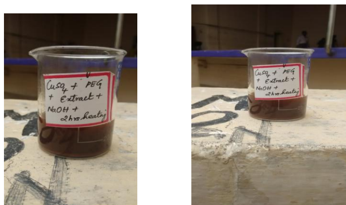
Fig 13: (a and b) Photograph of dispersion of copper nanoparticles taken before and after storage.
