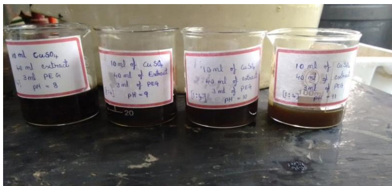
Fig.11: Photograph of formation of copper nanoparticles at different pH.
