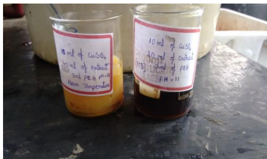
Fig.5: Photograph of formation of CuNPs at different temperature
