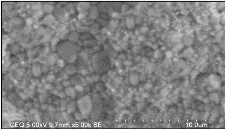
**Fig. 4. SEM analysis of Magnetite nanoparticles synthesized from  $\text{FeCl}_2$**
