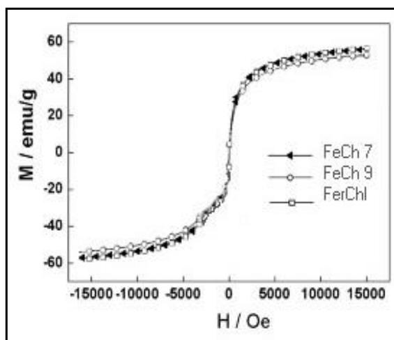
**Fig. 3. Ferromagnetism measurement for Magnetite nanoparticles synthesized from FeCl<sub>2</sub>**
