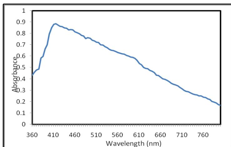
**Fig.6. UV-Vis absorbance spectrum of Magnetite nanoparticles synthesized from  $\text{FeCl}_2$**
