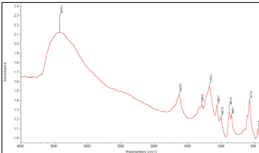
**Fig. 5. FTIR Spectrophotometer analysis of Magnetite nanoparticles synthesized from  $\text{FeCl}_2$**
