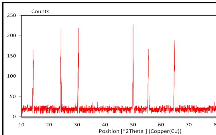
**Fig. 2. XRD spectral analysis for Magnetite nanoparticles synthesized from FeCl<sub>2</sub>**
