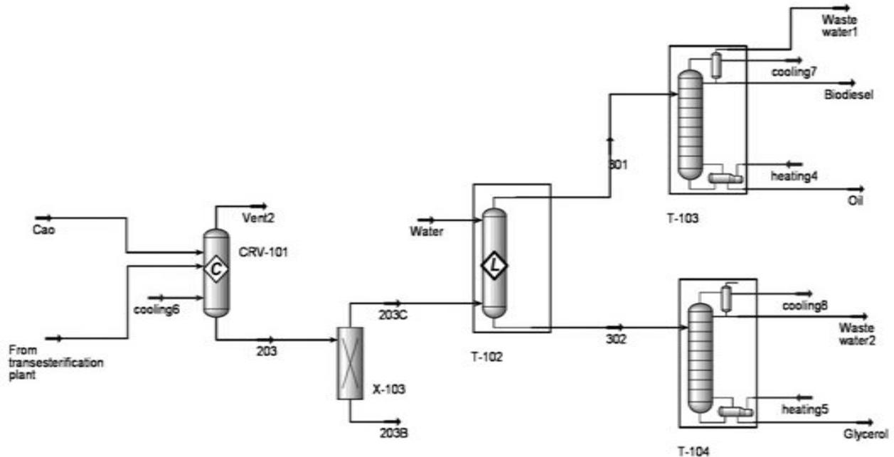
**Figure 8: Product purification flow sheet; where (CRV-101) neutralization tank, (X-103) settling tank, (T-102) water washing tower, (T-103) biodiesel purification distillation tower and (T-104) glycerol purification distillation tower.**
