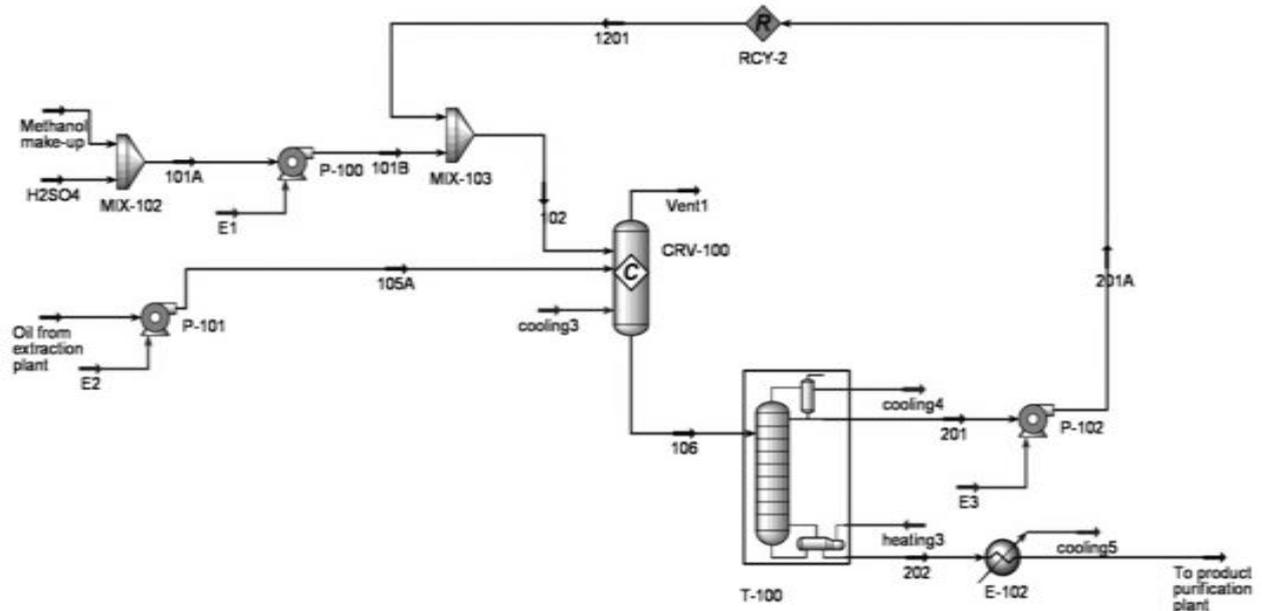
**Figure 7: Transesterification flow sheet; where (MIX-102) make-up alcohol/catalyst mixer, (MIX-103) recycled alcohol/catalyst and fresh alcohol mixer, (P-100) alcohol and catalyst pump, (P-101) oil pump, (P-102) recycled alcohol pump, (CRV-100) transesterification reactor, (T-100) methanol recovery distillation tower and (E-102) cooler.**
