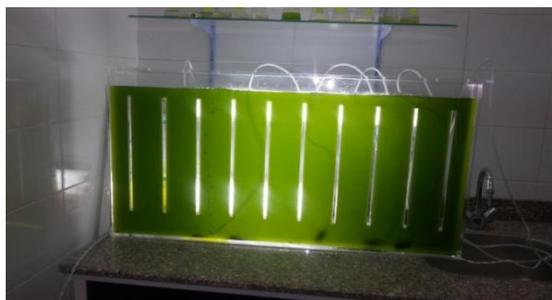
Figure 1: Newly installed Flat Panel Photo-bioreactor
