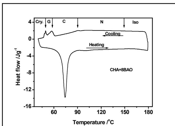
**Figure 7 DSC thermogram of CHA +8BAO hydrogen bonded complex**
