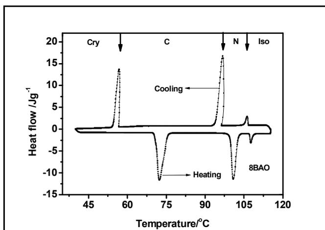
**Figure 6 DSC thermogram of pure 4 - octyloxy benzoic acid**
