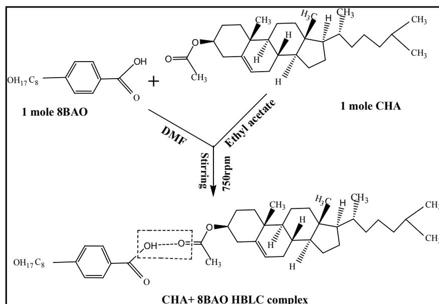
Figure 1 Molecular structure of CHA+8BAO hydrogen bonded complex
