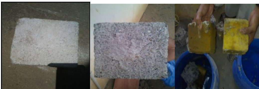
Fig.6 (a) Cube before immersion in acid, (b) Cube after immersion in H_2SO_4 and (c) Cubes after immersion in HCl.
