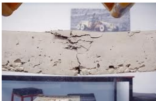
Fig 2.4 Failure Pattern Of flexural strength of beam Specimen
