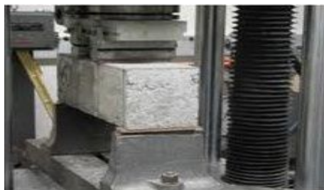
Fig 2.3 Experimental setup for flexural strength on concrete beam
