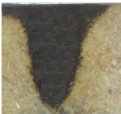
Fig. 3. Image of the key-hole of dray Swedish sample prepared at 36.5 W.
