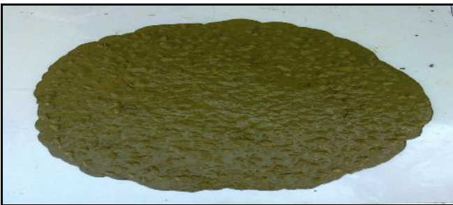
Fig 3: Slump flow test
