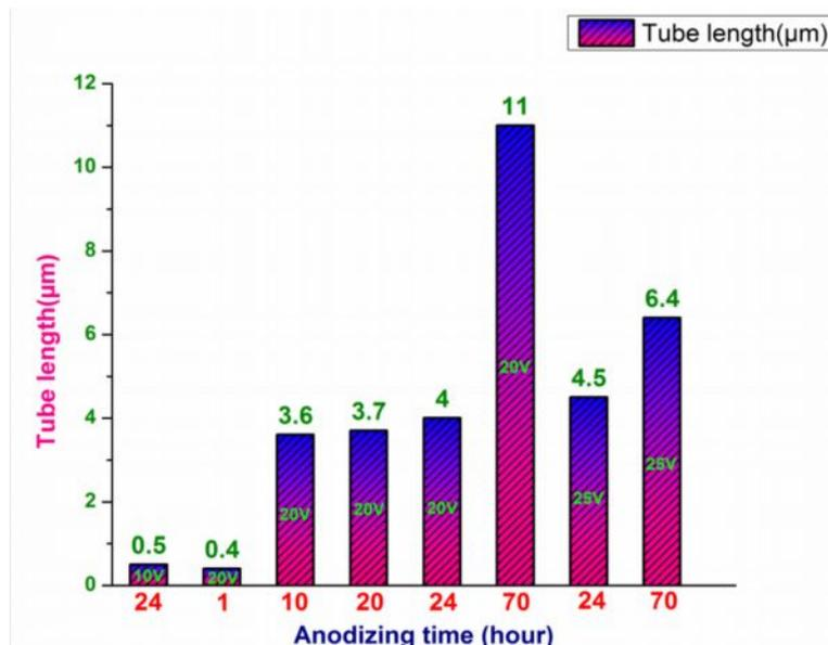
Fig. 3 Reported  $\text{TiO}_2$  nanotubes synthesized at different voltage -ref [22]
