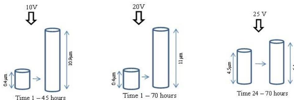
**Fig. 6. Optimized growth prediction of TiO<sub>2</sub> nanotube length for various voltages**
