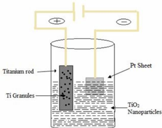
Fig. 2 Anodization of Ti foils to form  $\text{TiO}_2$  nanotubes
