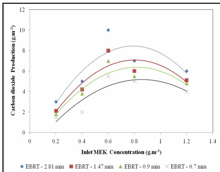
Fig 4 Effect of inlet MEK concentration on carbon dioxide production at various gas flow rates.
