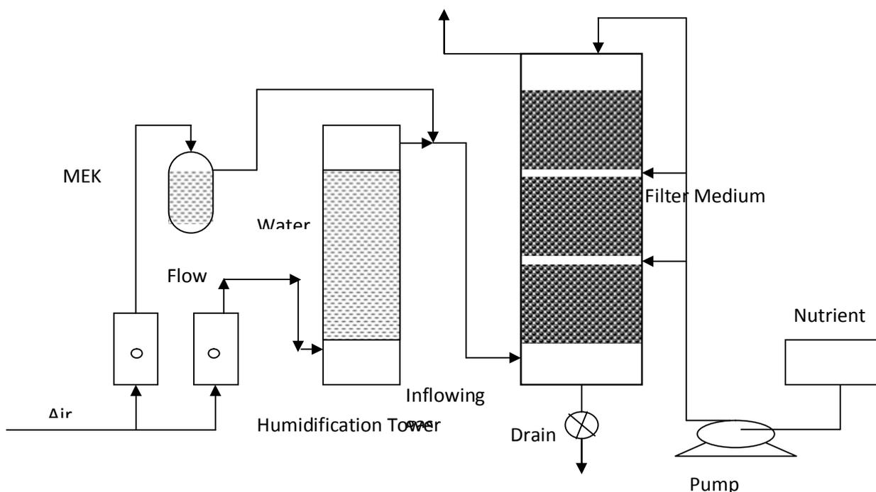
**Fig. 1. Schematic diagram of up flow biofilter system**
