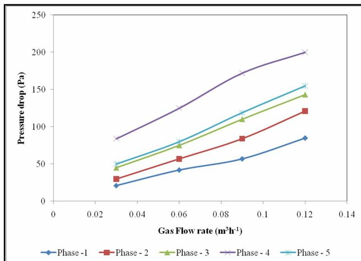
**Fig 7 Effect of pressure drop on the different gas flow rate for cornstalk and pressmud based biofilter for the removal of MEK**
