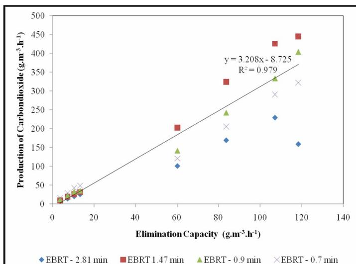
**Fig 5 Profile of carbon dioxide production rate at different inlet concentration during the removal of MEK**
