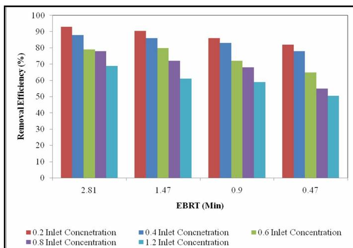
**Fig 3 Shows the effect of EBRT on the removal efficiency**
