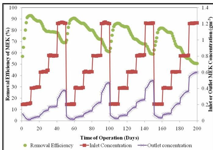
**Fig. 2. Start-up of the biofilter for the removal of MEK using pressmud and corn stack based biofilter**
