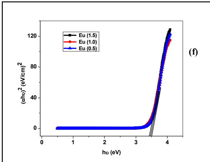
**Fig. 2**  $(\alpha hv)^2$  Vs photon energy plots of (d) Sm (1.0, 1.5, and 2.0) (e) Dy (1.0, 1.5, and 2.0) & (f) Eu (0.5, 1.0, and 1.5) doped borate glasses
