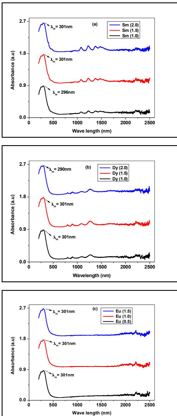
**Fig. 1** Absorption spectra of (a) Sm (1.0, 1.5, and 2.0) (b) Dy (1.0, 1.5, and 2.0) & (c) Eu (0.5, 1.0, and 1.5) doped borate glasses
