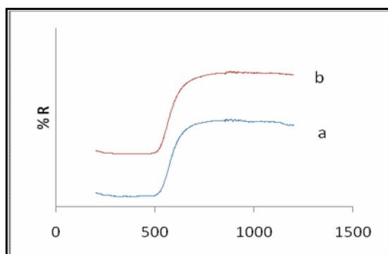
Fig. 6. UV spectra (reflectance) of CdS Bulk (a), CdS QD (b)
