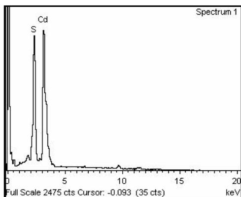
**Fig. 3. EDX pattern of CdS Nanoparticle**
