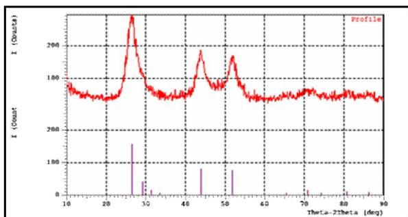
**Fig. 1. X-ray diffraction pattern of CdS Nanoparticle**
