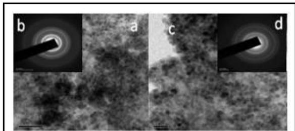
Fig. 4. HRTEM images of CdS QD (a, c) and SAED images of CdS QD (b, d)
