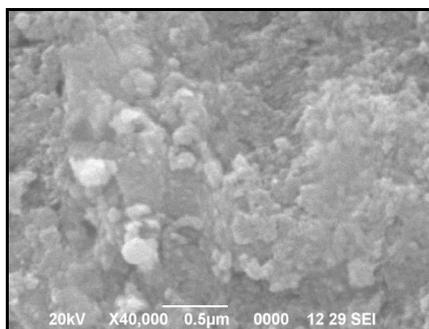
**Fig. 2. SEM image of CdS nanoparticle**
