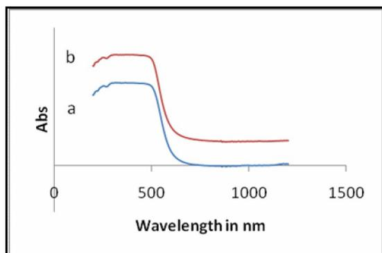
Fig. 5. UV spectra (absorbance) of CdS Bulk (a), CdS nanoparticle (b)
