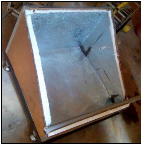
Fig. 1. Single slope solar still
