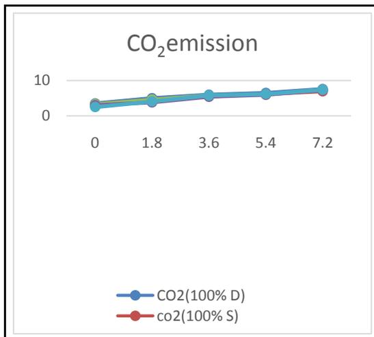
**Fig. 4(a)**The variation in CO<sub>2</sub> with different load conditions In Cases IV hydrogen shows
