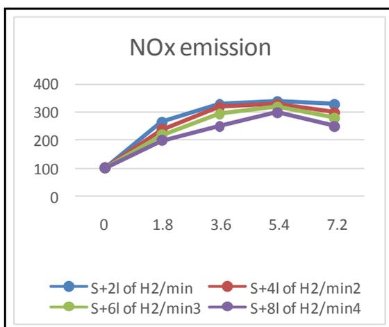
**Fig. 6(b)** The variation in  $NO_x$  with different load conditions
