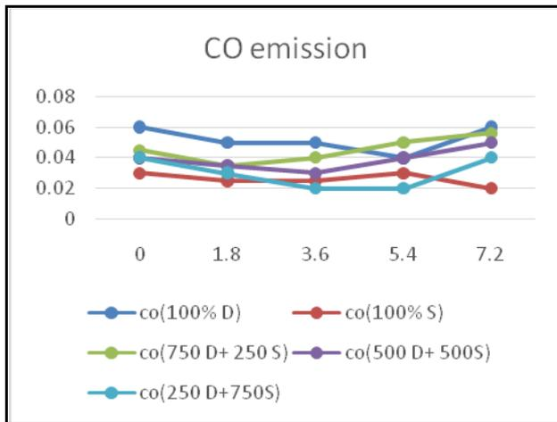
**Fig. 3(a)The variation in CO with different load conditions**
