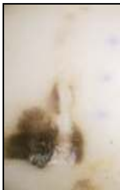
Figure 5. Eroded Silicone rubber with track length of 35mm
