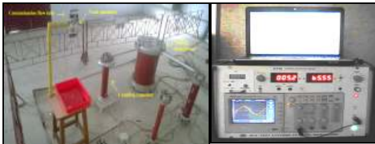
Figure 3. photograph of IPT test setup and PD measurement system
