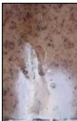
Figure 9. Eroded silicone rubber with silica nanoparticles with track length of 27mm
