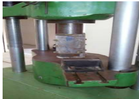
Figure 4b: Experimental setup for push out test
