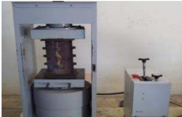
Figure 4a: Experimental setup for Axial compressions
