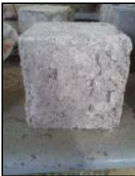
Fig.4 Sample Picture of specimen after curing in NaCl
