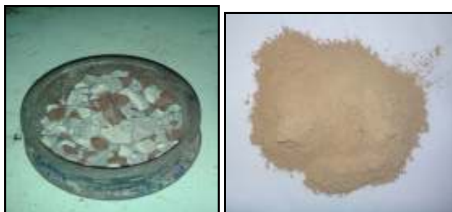
Fig. 1 Ceramic material before and after grinding in Ball Mill
