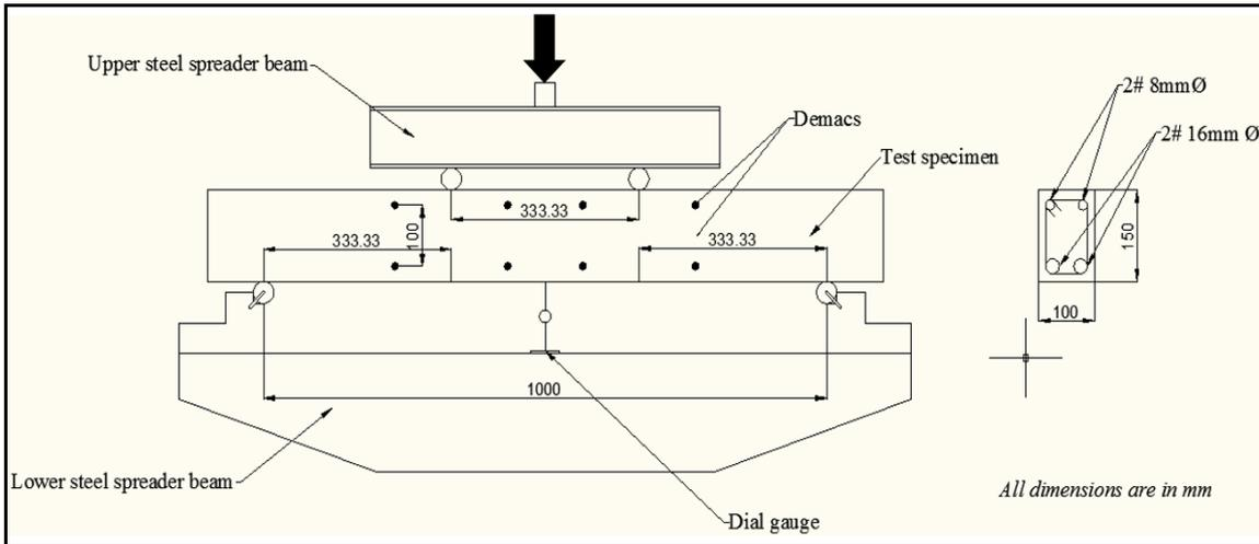
**Fig.3 Test setup and reinforcement details**
