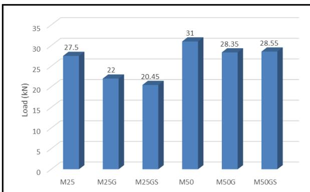
**Fig.13 First crack load**
