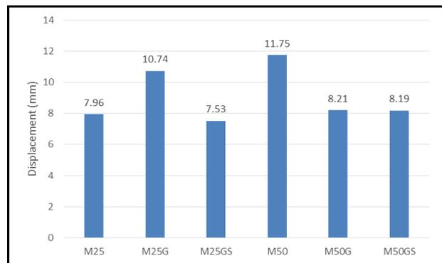
**Fig.12 Maximum displacement of beams**
