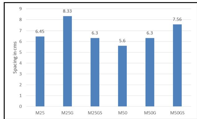
**Fig.10 Average spacing between the cracks**
