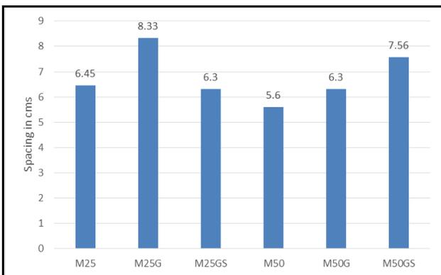
**Fig.11 Average spacing between the cracks**
