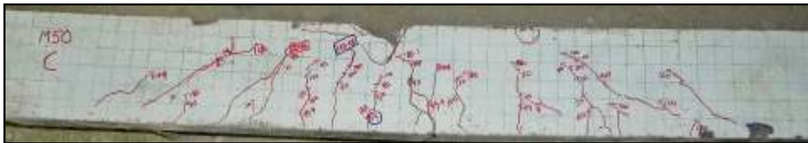
c. Crack pattern for M50 control beam
