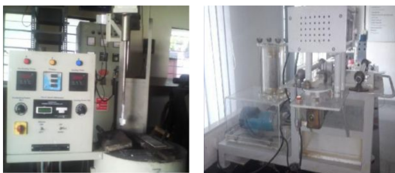
Figure 1. Stir Casting Set up
